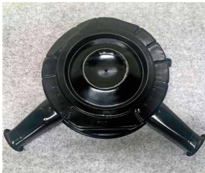
Air filter after powder coating
