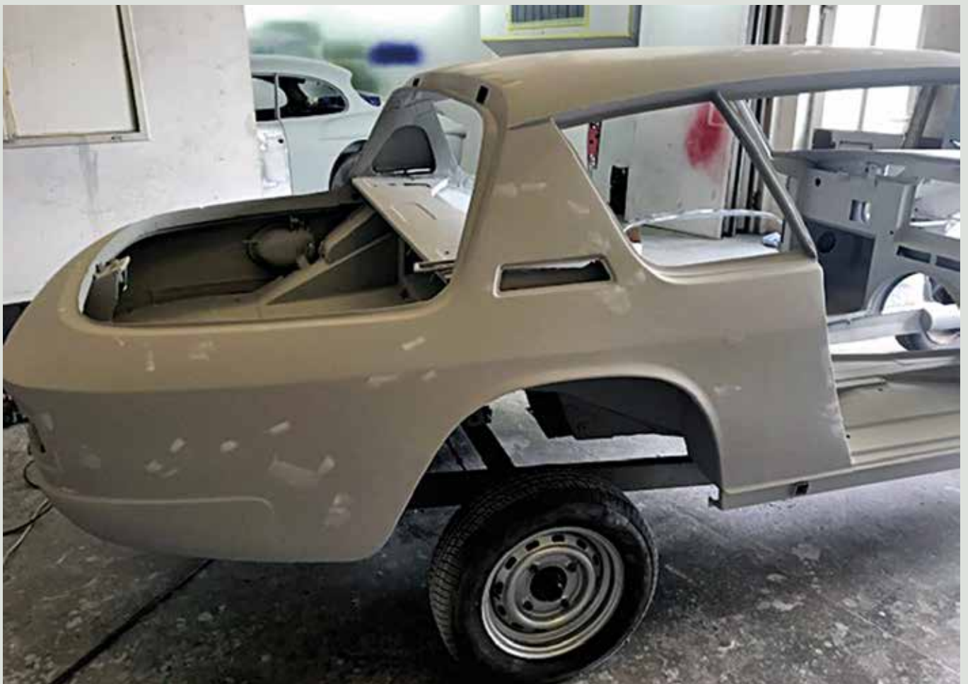
New arch fettled and painted
