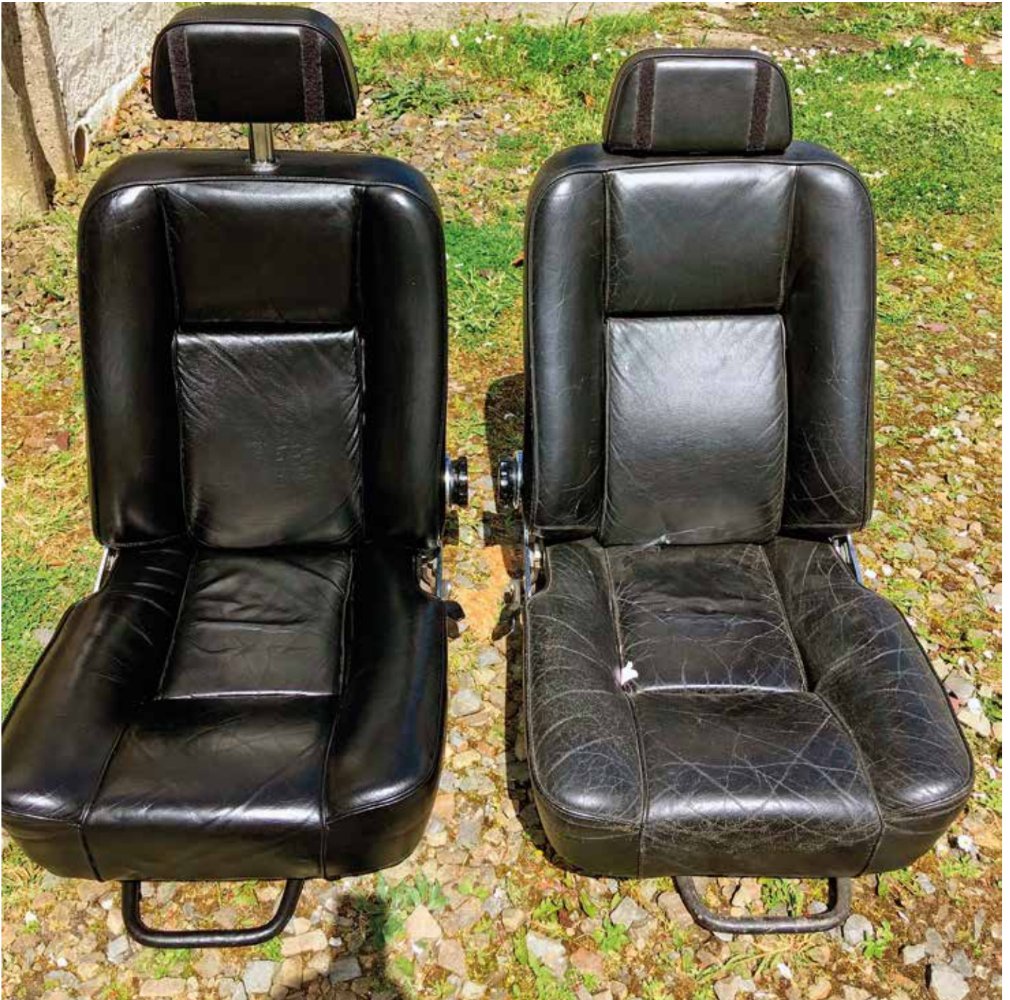
The driver's seat was much worse than the seat on the left before recolouring
