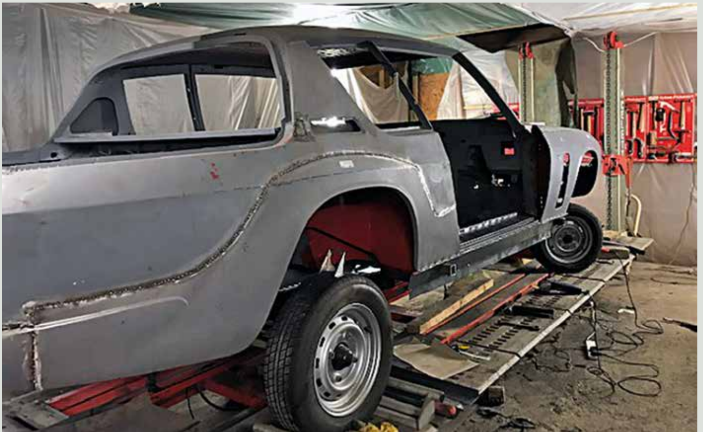
New arch welded in place
