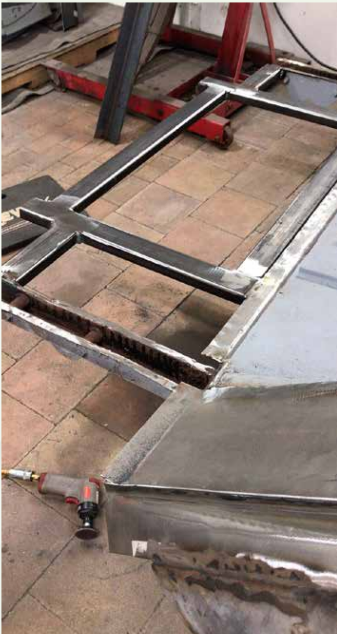
The rear end of the SP being rebuilt and modified for crash-worthiness
