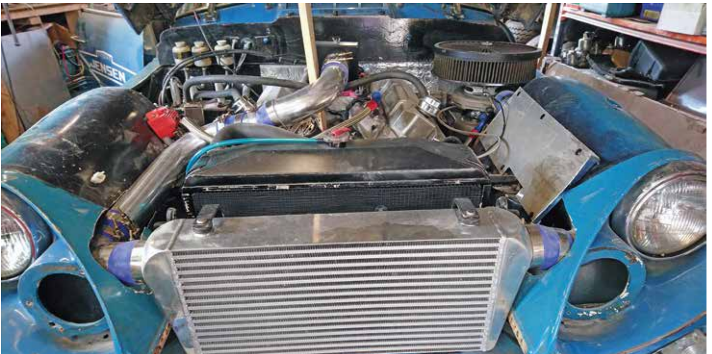
The engine (modified by John Sleath and now of 8.2 litre capacity) - checking for fit with the massive turbocharger, intercooler and radiator
