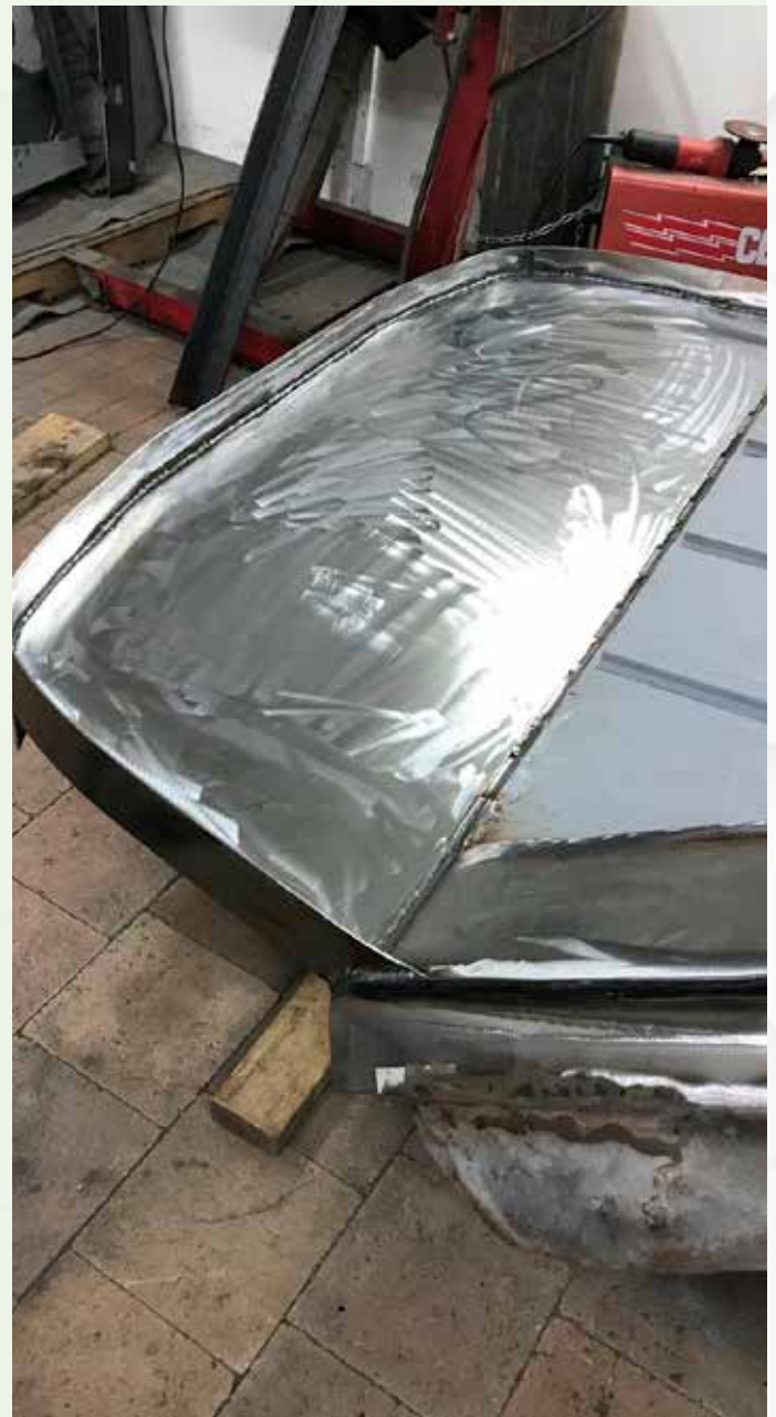
The rear end of the SP being rebuilt and modified for crash-worthiness
