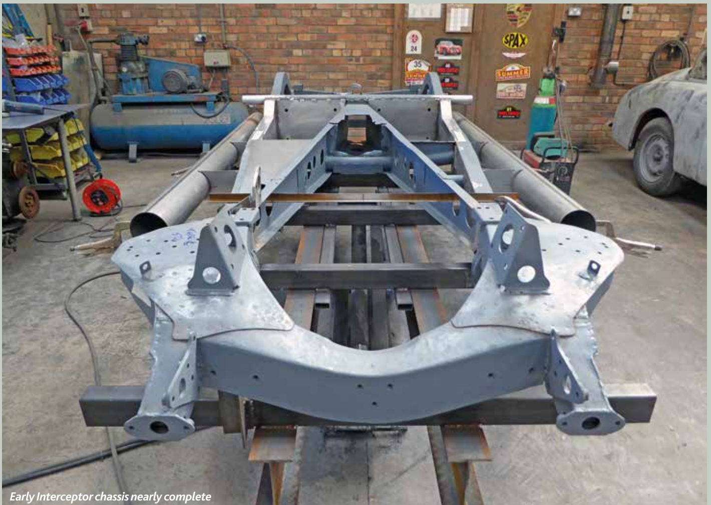
Early Interceptor modified chassis rails nearly complete
