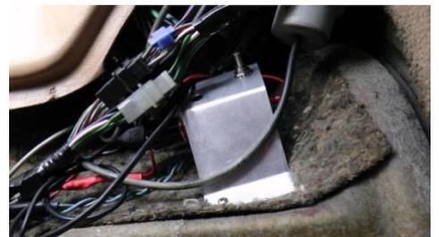
Figure 5 New bracket assembly installed in car
